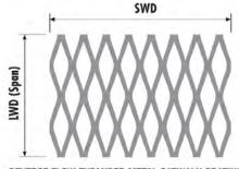
REVERSE FLOW EXPANDED METAL CATWALK GRATING
