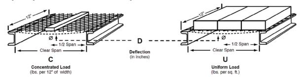
**Clear Span:** The distance between supports, measured from the inside edge of one support to the inside edge of the next support.
