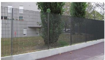
not joined nor welded side by side, with a height of ... inch, width 6'-6 27/64", mesh size 2 7/16" x 5 13/64" with 63/64" x 1/8" vertical flat bars (centers distance 2 7/16") and 11/64" diameter horizontal round bars (centers distance
