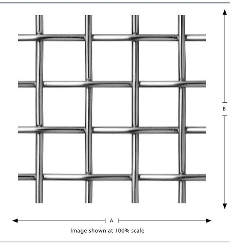
**Mesh Category:** Mid-Fill 70.1 % **Percent Open Area:** Weight: 1.70 lbs/sq ft Crimp Style\*: **PLPL** Maximum "A" Dimension: 240 inches Maximum "B" Dimension: 120 inches Opening Limitation\*\*: 0.838 inches **Overall Thickness:** 0.320 inches **Aspect Ratio:** 1.00:1 **Available Alloys:** Stainless, Bronze
