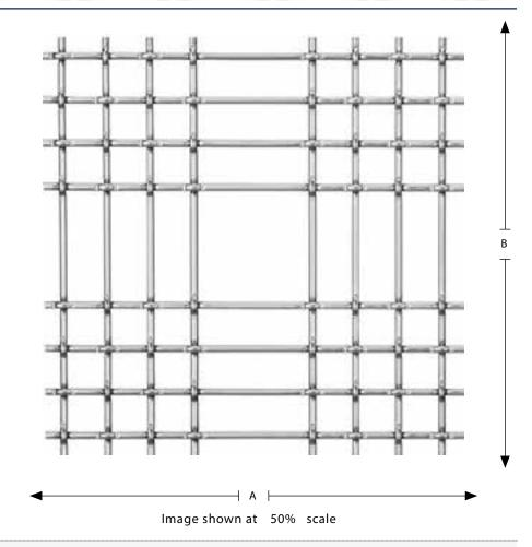
**Mesh Category:** Large **Percent Open Area:** 77.4 % Weight: 1.04 lbs/sq ft **Crimp Style\*:** 4L4L Maximum "A" Dimension: 240 inches Maximum "B" Dimension: 120 inches Opening Limitation\*\*: 2.10 inches **Overall Thickness:** 0.255 inches **Aspect Ratio:** 1.00:1 Stainless, Mild Steel, Aluminum, Copper, Bronze, Brass, Pre-Galv, Galfan **Available Alloys:**
