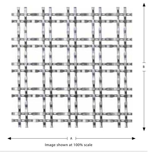
**Mesh Category:** Mid-Fill **Percent Open Area:** 61 % Weight: 1.00 lbs/sq ft **Crimp Style\*:** 2F2F Maximum "A" Dimension: 240 inches Maximum "B" Dimension: 120 inches Opening Limitation\*\*: 0.50 inches **Overall Thickness:** 0.13 inches **Aspect Ratio:** 1.00:1 **Available Alloys:** Stainless, Mild Steel, Bronze, Pre-Galv
