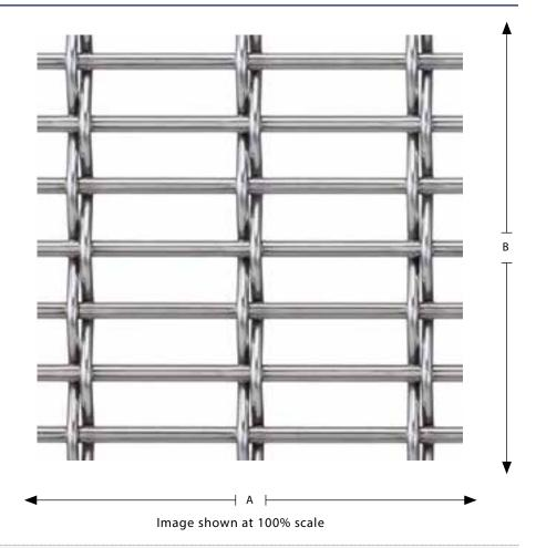
**Mesh Category:** Mid-Fill **Percent Open Area:** 61.7 % Weight: 2.12 lbs/sq ft PS2PZ **Crimp Style\*:** Maximum "A" Dimension: 240 inches Maximum "B" Dimension: 120 inches Opening Limitation\*\*: 0.471 inches **Overall Thickness:** 0.390 inches 2.67:1 **Aspect Ratio:** Stainless, Aluminum, Mild Steel, Copper, Bronze, Brass, Pre-Galv, Galfan **Available Alloys:**
