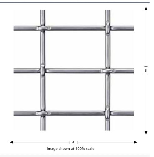
**Mesh Category:** Large **Percent Open Area:** 81.3 % Weight: 1.04 lbs/sq ft **Crimp Style\*: LCLCZ** Maximum "A" Dimension: 240 inches Maximum "B" Dimension: 120 inches Opening Limitation\*\*: 1.25 inches **Overall Thickness:** 0.324 inches **Aspect Ratio:** 1.62:1 Stainless, Plain Steel, Aluminum, Copper, Bronze, Brass, Pre-Galv, Galfan **Available Alloys:**
