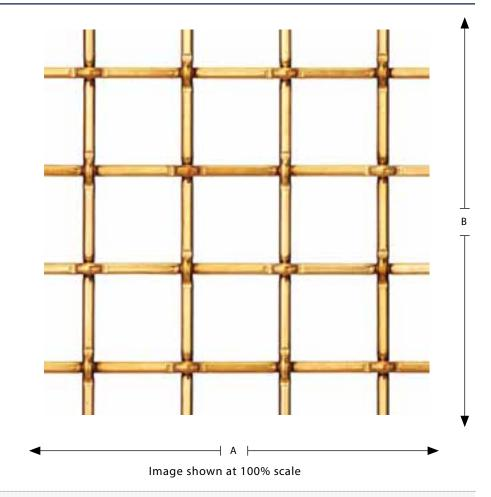
**Mesh Category:** Mid-Fill **Percent Open Area:** 77.4 % Weight: .928 lbs/sq ft **Crimp Style\*: LCLC** Maximum "A" Dimension: 1800 inches Maximum "B" Dimension: 120 inches Opening Limitation\*\*: .88 inches **Overall Thickness:** 0.240 inches **Aspect Ratio:** 1.00:1 Stainless, Mild Steel, Aluminum, Bronze, Brass, Copper, Pre-Galv, Galfan **Available Alloys:**
