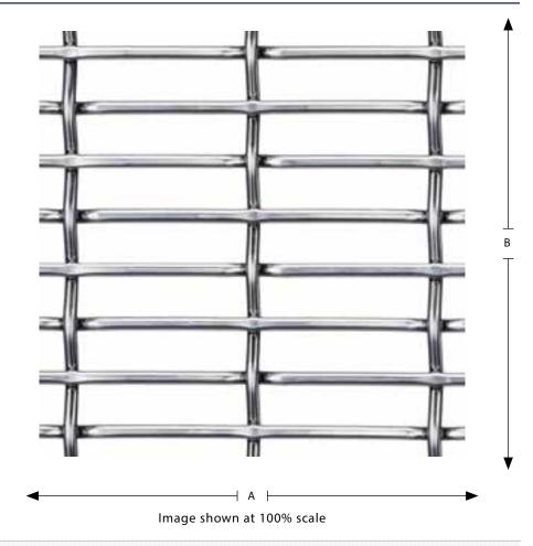
**Mesh Category:** Large **Percent Open Area:** 66.5 % Weight: 1.85 lbs/sq ft **Crimp Style\*: FTPLZ** Maximum "A" Dimension: 240 inches Maximum "B" Dimension: 120 inches Opening Limitation\*\*: 0.42 inches **Overall Thickness:** 0.285 inches 3.33:1 **Aspect Ratio:** Stainless, Mild Steel, Aluminum, Copper, Bronze, Brass, Pre-Galv, Galfan **Available Alloys:**
